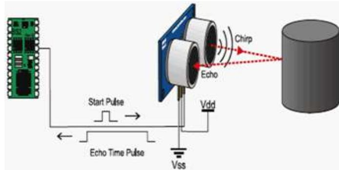
Figure 5. Ultrasonic detcting obstacle<sup>[6]</sup>
