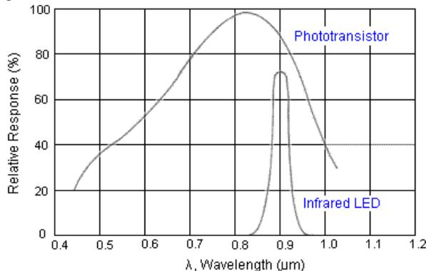
**Fig: Response of phototransistor and Infrared LED**
