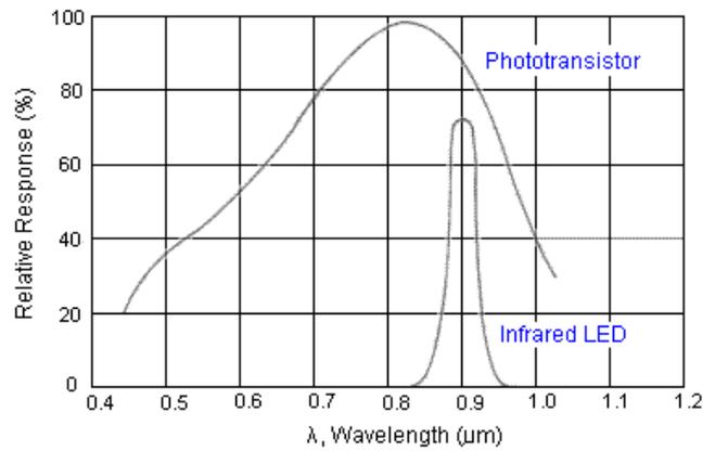
Fig: Responses of the phototransistor and Infrared LED
