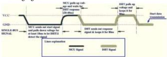
Fig: DHT11 signaling and working
