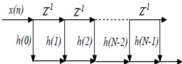
Fig.2: Convolution FIR filter structure
