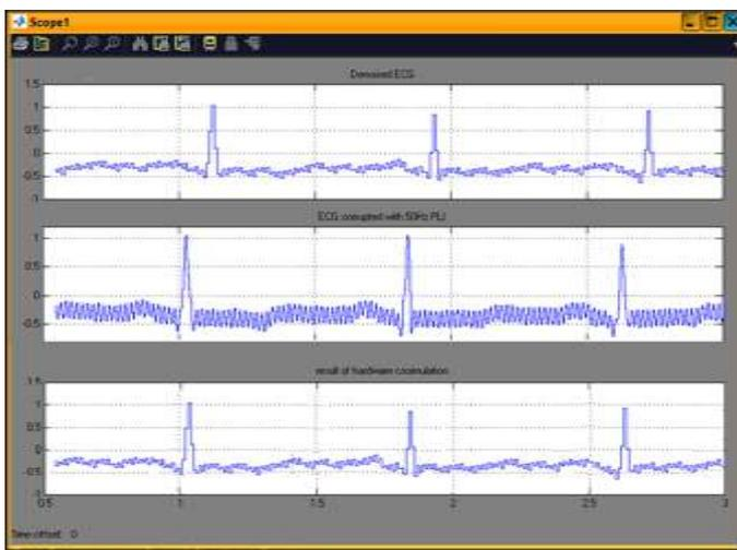
Fig.9: Results after Implementation on Spartan 3E Device.
