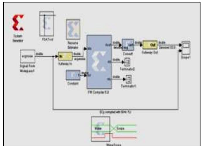
Fig. 5: Simulink model for Distributed arithmetic based FIR filter design using FIR Compiler 5.0
