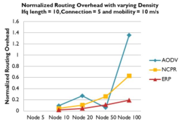
Fig. 1 Normalized Routing Overhead vs Node Density
