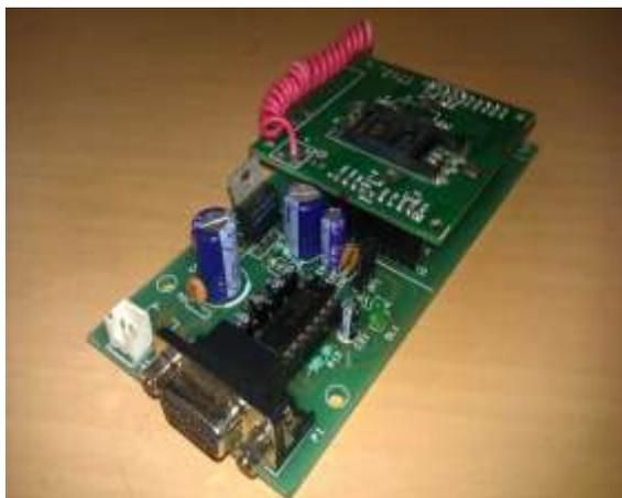
Figure.4 GSM Module
