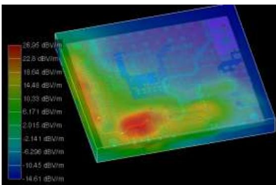
Fig.2 E field radiation from bad board at 1GHz
