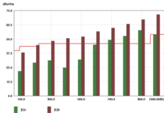
Fig.1 Emissions from bad board (failing FCC class A limits)
