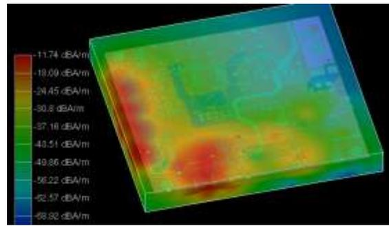
Fig.3 H field radiation from bad board at 1GHz
