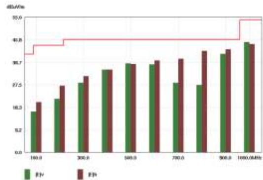
Fig.4 Reduced emission from good board (passing FCC class B limits)
