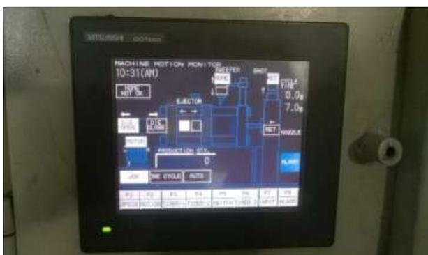
Fig.3: Front Panel Monitor Of GOT1000
