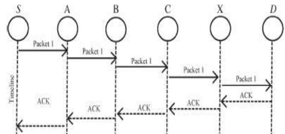
Figure 2: ACK (An End-End Acknowledgement)
