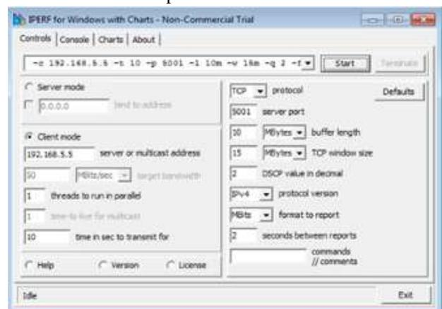
Fig. 1 IPERF (GUI Based Version)
