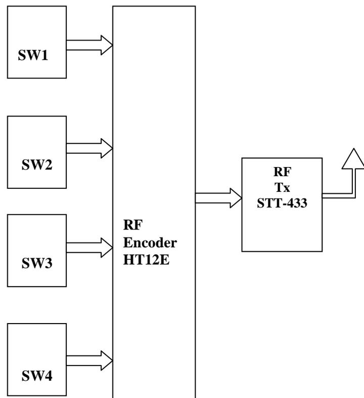
Fig1: Transmitter Module
