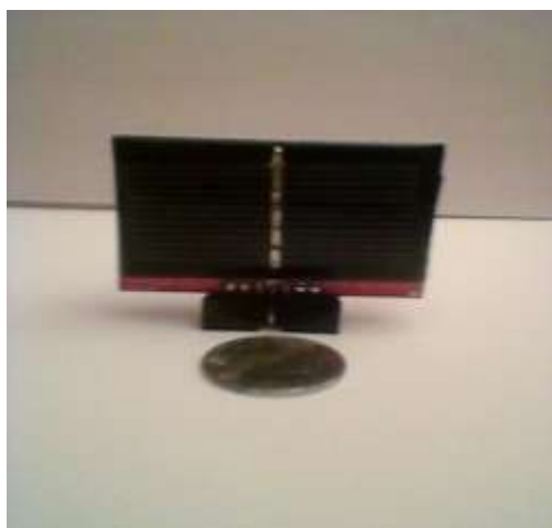
Figure 3 Tiny solar unit for recharging WSN node
