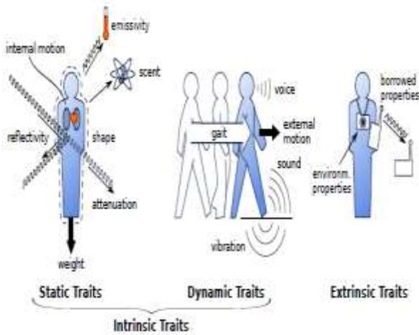
Fig. 1. Physical traits used by motion sensors.
