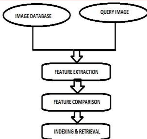
Figure 1. Block Diagram Of CBIR System
