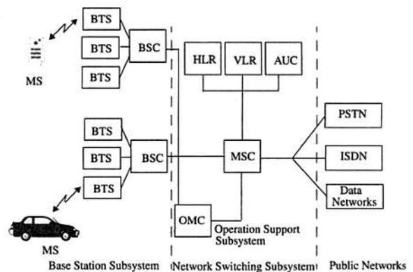
Figure1:- GSM Architecture
