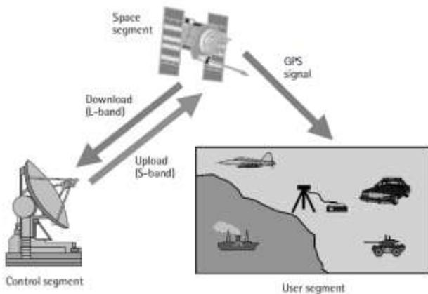
Figure 2:- Three segments of GPS
