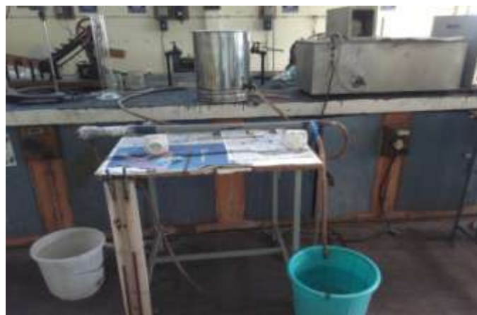
Figure 1. Fabricated Double Pipe Heat Exchanger Experimental Setup
