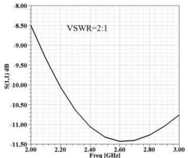
Figure 5. S-Parameter v/s Frequency of Subsidiary Antenna.
