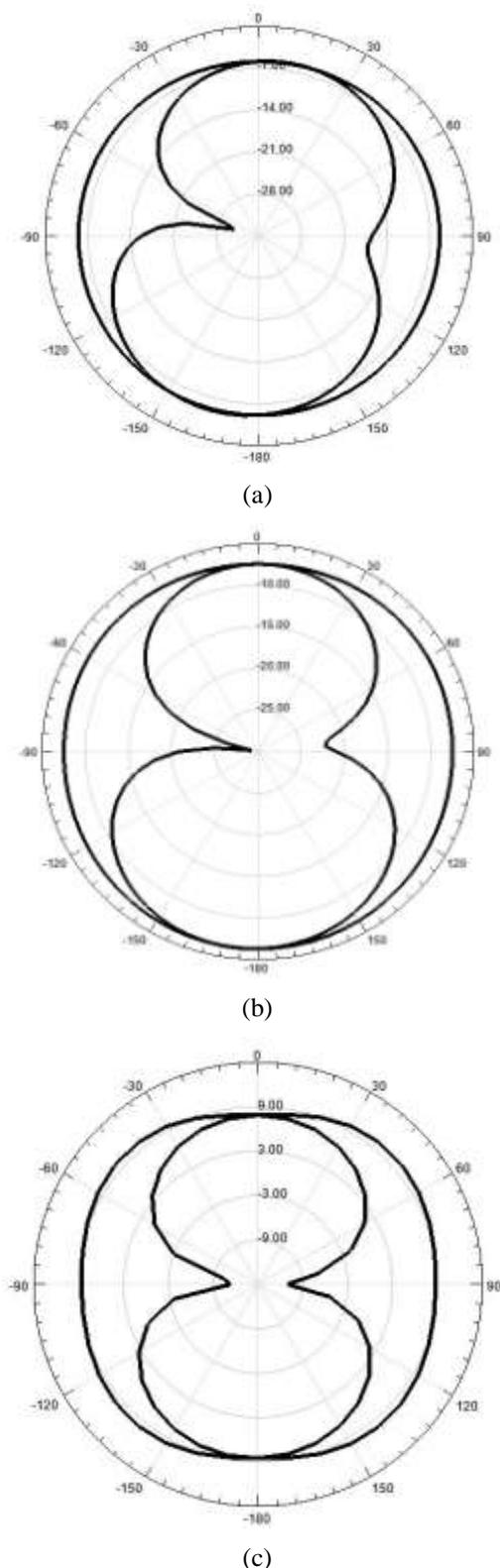
Figure 6. Radiation plots of (a) Main Antenna at 1 GHz (b) Main Antenna at 1.5GHz (c) Subsidiary Antenna at 2.5 GHz.
