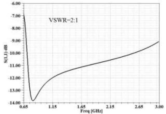
Figure 4. S-Parameter v/s Frequency of Main Antenna.
