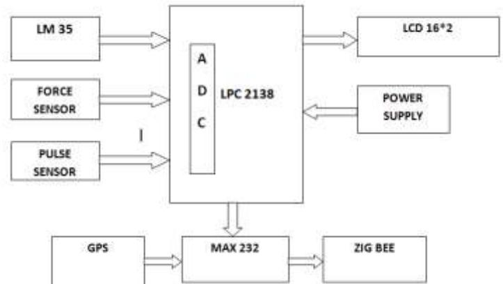
Figure.2 Block Diagram of Slave
