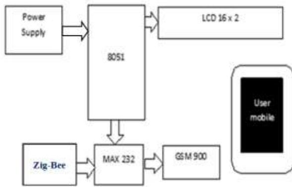
Figure.3 Block Diagram of Master
