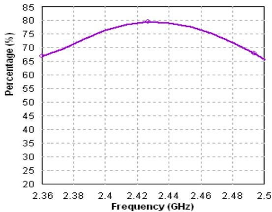
Fig.7. Antenna efficiency Vs frequency
