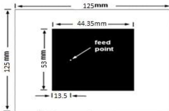
Fig.2. Geometry of top view the high gain Microstrip Rectangular patch Antenna
