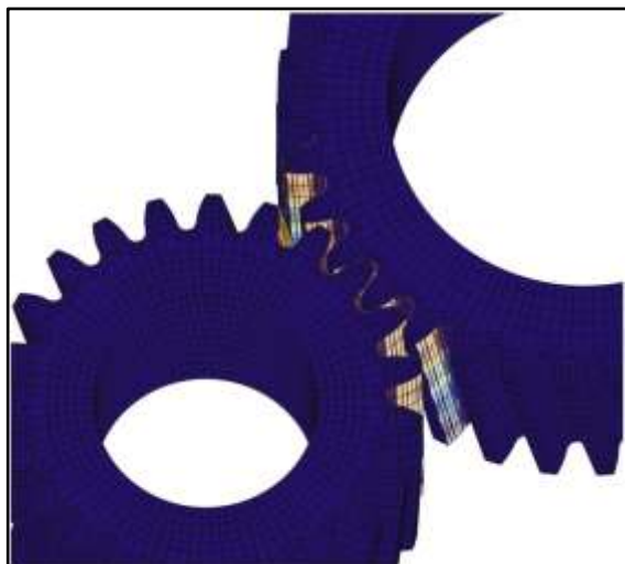
Fig4. 3D finite element model prior to refinement
