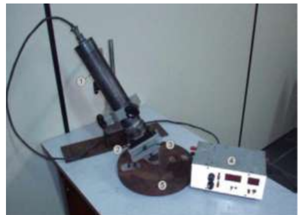
Fig 1. General view of the portable X-ray apparatus: 1-high voltage source; 2-X-ray tube; 3-collimator-cassette unit; 4-control unit; 5-analysed sample [18].
