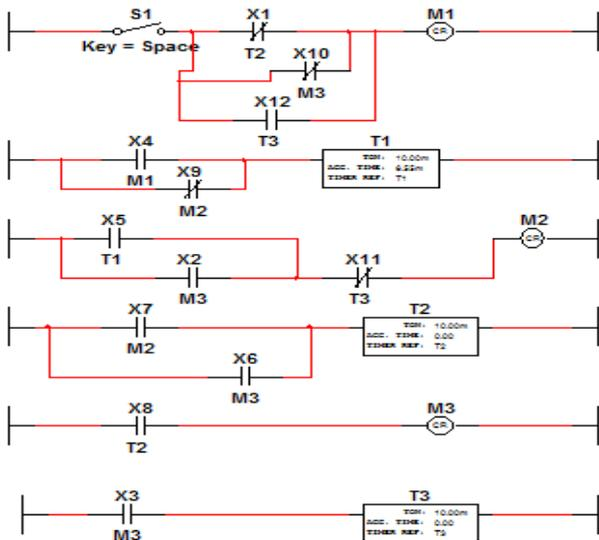
Figure 8: RLL with switch off condition
