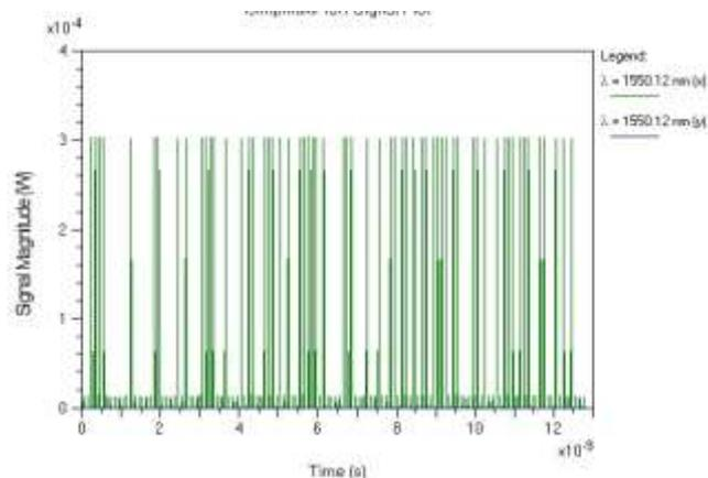
Fig.5 Downstream signal after 117 km
