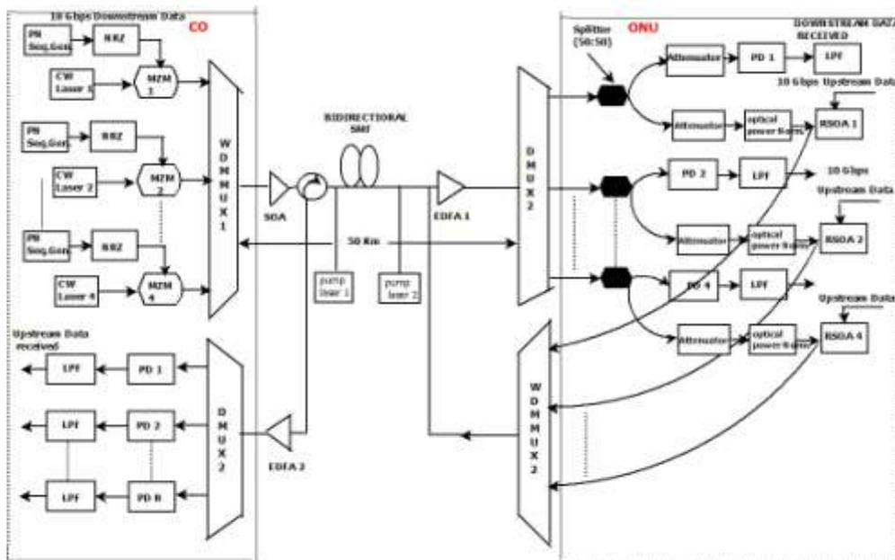
Fig.2.Experimental set-up for proposed scheme
