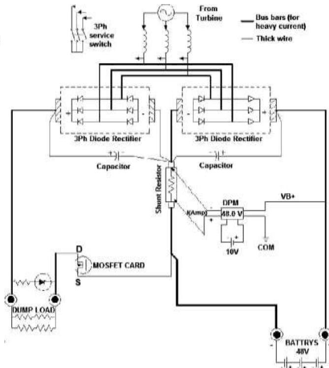
Fig. 3 Wind charge controller’s internal blocks
