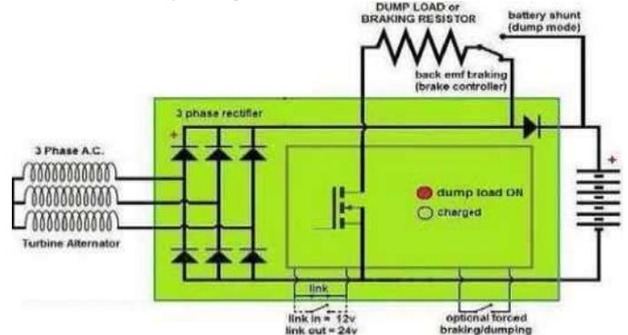
Fig. 6 MOSFET as switch for controlling switching of dump load
