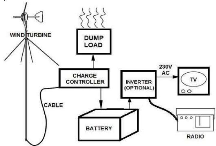
Fig. 1 Block diagram of wind energy system
