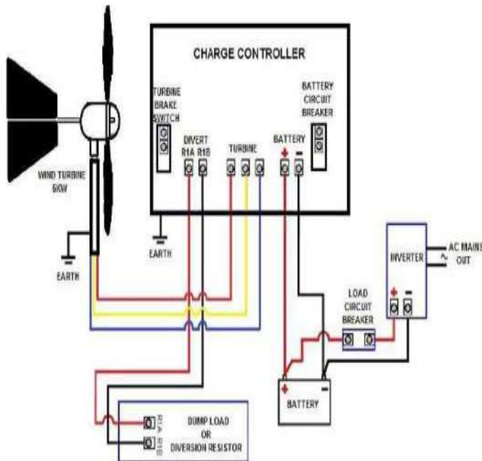
Fig. 2 Wind charge controller connected to dumpload and battery
