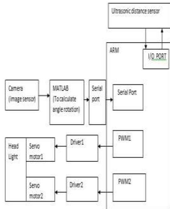
Figure 3: Block Diagram of proposed design
