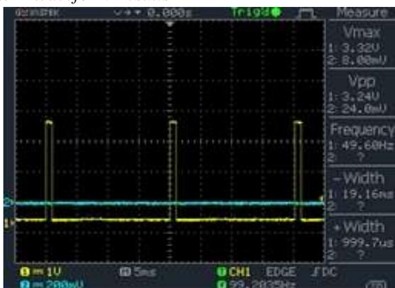
Figure 7: PWM waveform with 1ms + width
