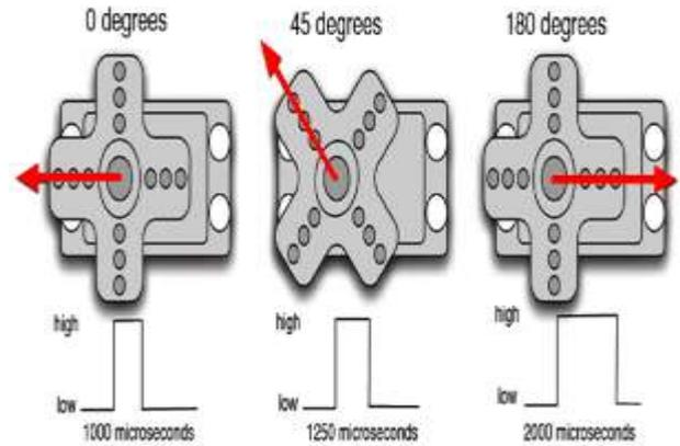
Figure.4 : PWM (Pulse Width Modulation)
