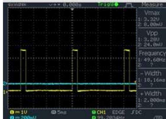
Figure 8: PWM waveform with 2ms + width
