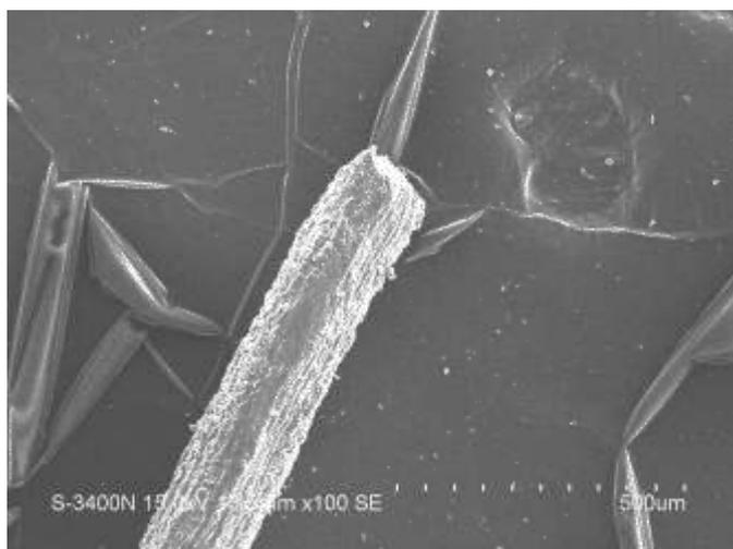
Fig.2 SEM image of fractured fiber after tensile test
