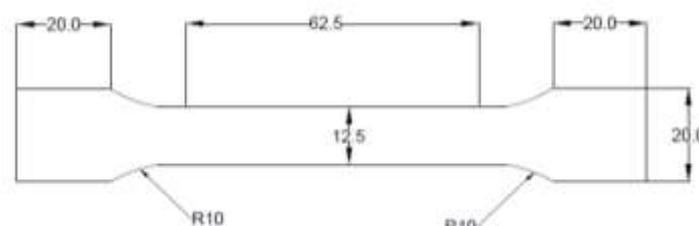
Fig.1 Dimensions of tensile test specimen
