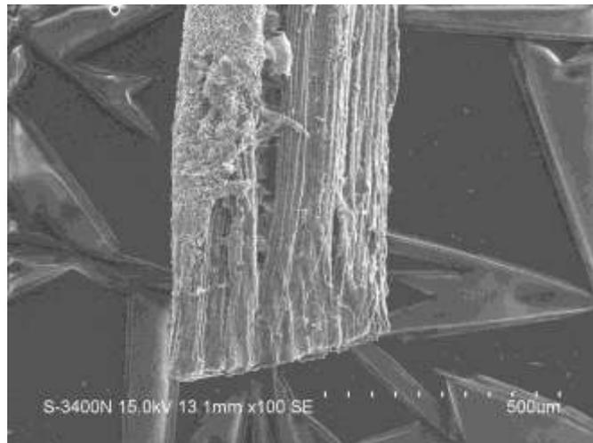
Fig.3 SEM image of fractured fiber after flexural test
