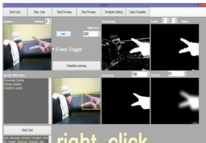
Figure 4: User Interface and hand gesture being identified and matched to the template "right\_click"
