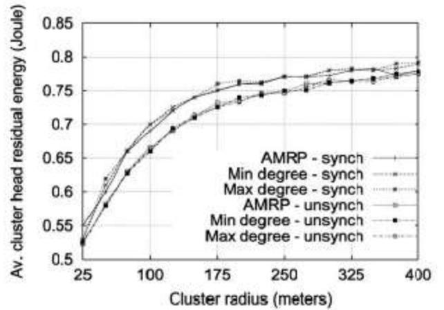
Fig 6: HEED average cluster head energy for synchronized and pseudo synchronized nodes (graph is simulation result of [2])
