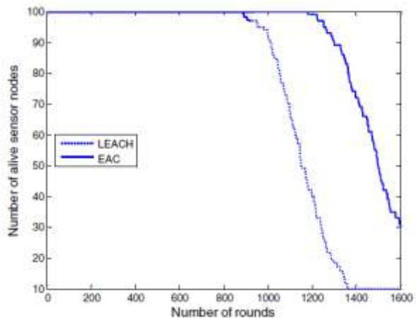
Fig 7: comparison of network lifetime (graph is a simulation result of [9])
