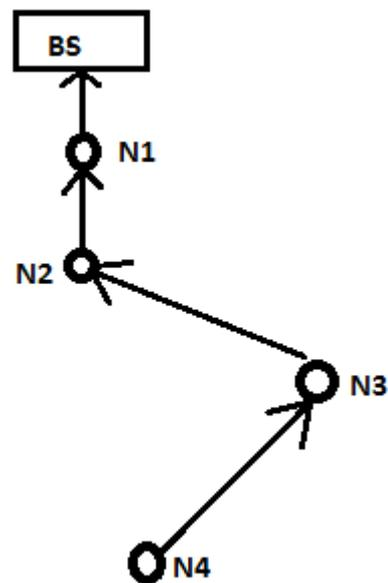
Fig 3: flow of data in chain to B.S
