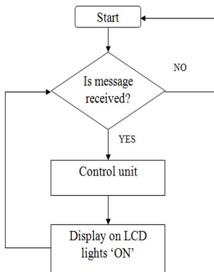
The receiver is located at the control room. As the message from the transmitter section is received by the control room it is immediately displayed on the LCD. This helps to monitor the status of tunnel lights and railway gate from the control room. A key is available in the control room to order lights on or off in the tunnel in the absence of train. This key signal is checked at the transmitter section.[4]
