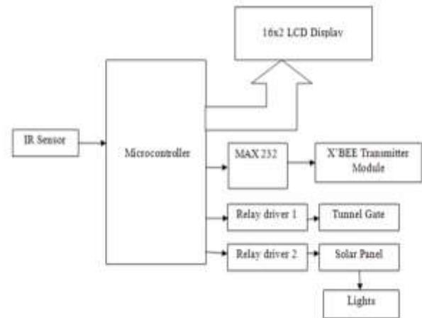
Fig 1. Transmitter section
