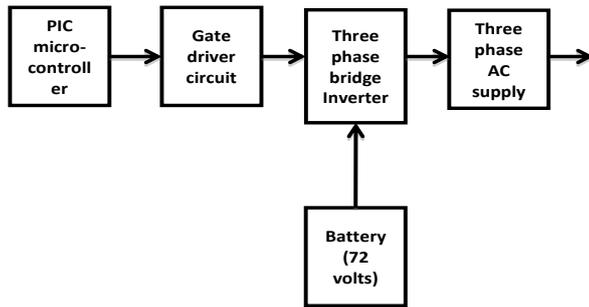
Figure:-1 Block diagram of Hardware implemented system
