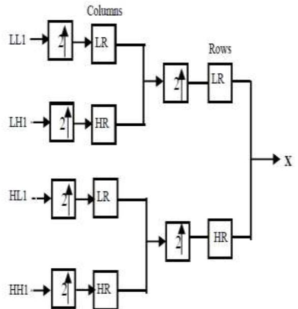
Figure 2 Wavelet filter bank of one level image-Reconstruction
