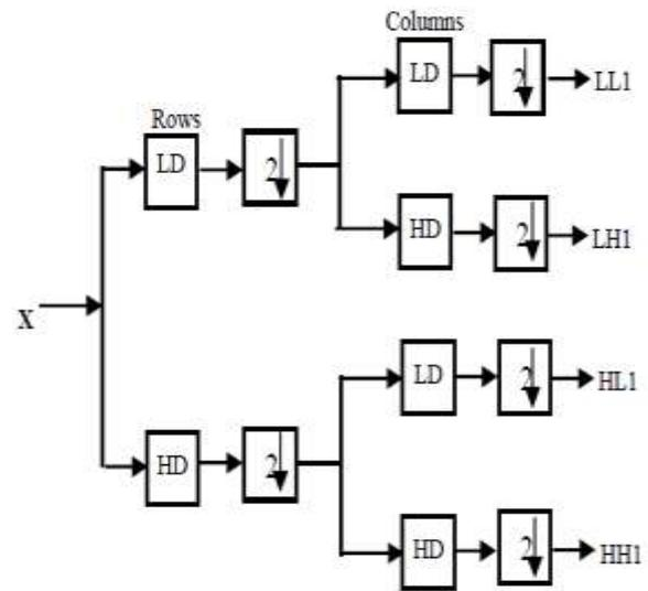
Figure .1 Wavelet filter bank of one level image-decomposition
