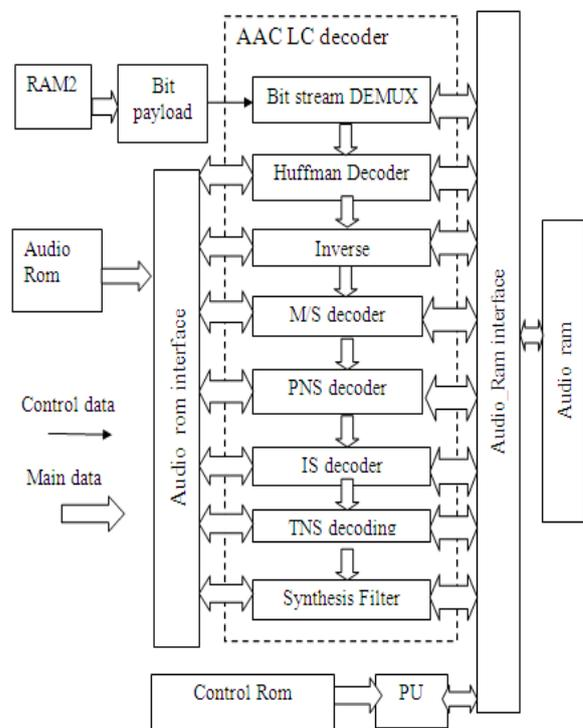
**Figure 3: Block Diagram of AAC LC Decoder**
