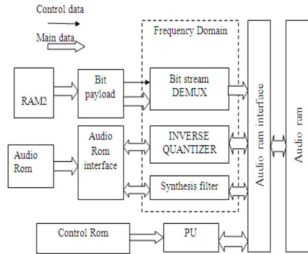
**Figure 2: Block Diagram of MP2 Decoder**
