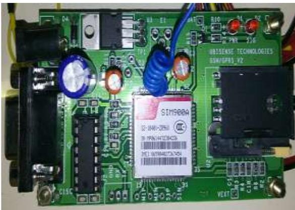
Figure 4 GSM Module
