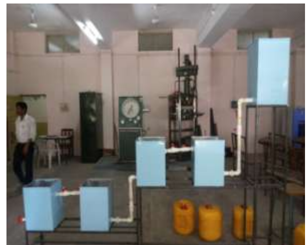
Fig 2 :- integrated grey water treatment plant
