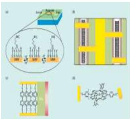
(a) Silicon nanowire that detect pH, (b) Carbon Nanotube, (c) Small Organic molecules, and (d) Biomolecules, are examples of material, devices and circuits that could be used for pollutant sensing, prevention and treatment.
