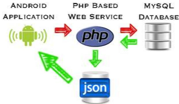
Figure 3. Application Communication Architecture [4]
