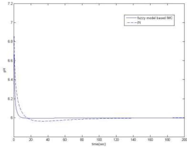
Fig 6. Servo response for pH change from pH 7 to pH 6
