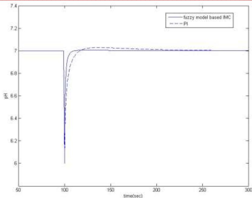
Fig 12. Regulatory response for disturbance of -1 pH
