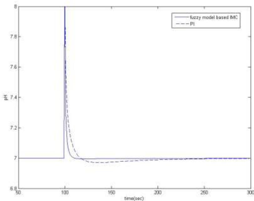
Fig 11. Regulatory response for disturbance of +1 pH
