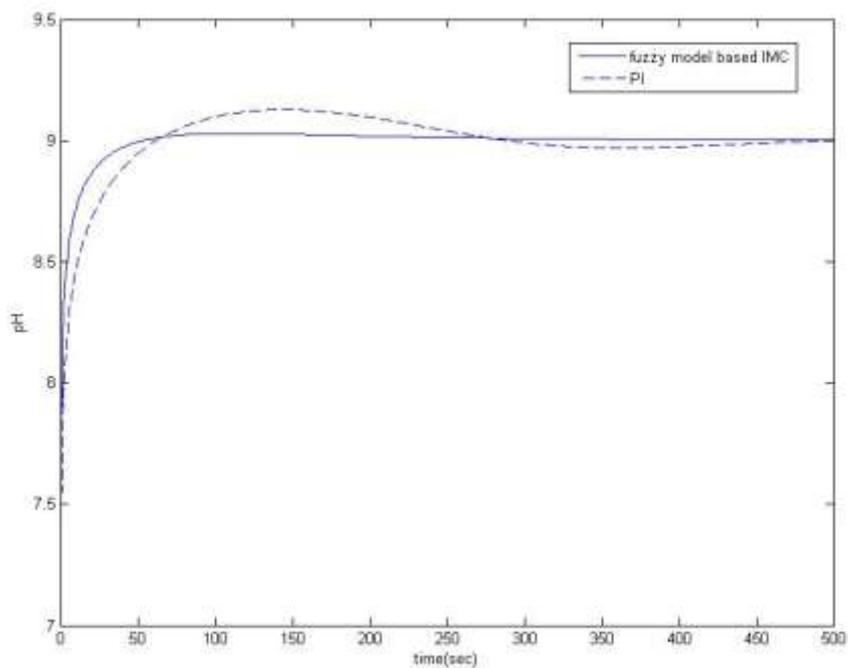
Fig 8. Servo response for pH change from pH 7 to pH 9
