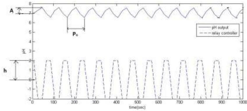
Fig 5. Relay feedback test for pH process
