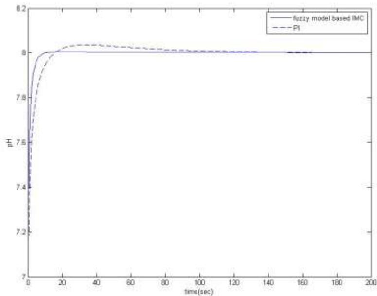
Fig 7. Servo response for pH change from pH 7 to pH 8
