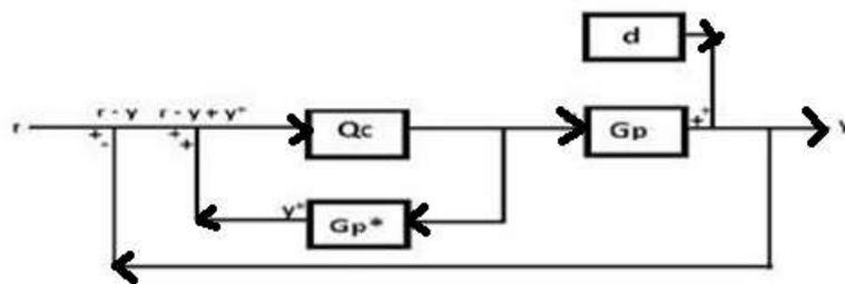
Fig 3. Block diagram of IMC based PI controller
