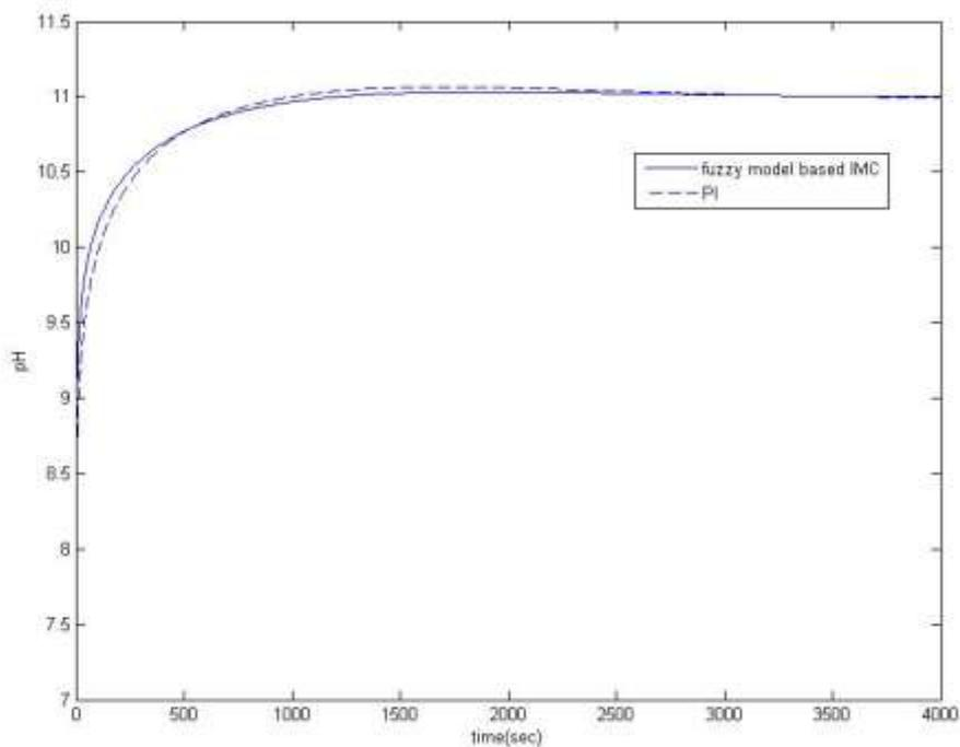
Fig 9. Servo response for pH change from pH 7 to pH 11
