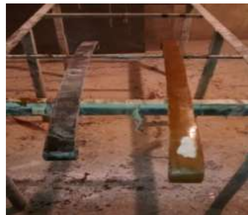
Fig.9 Steel and E-glass epoxy spring
