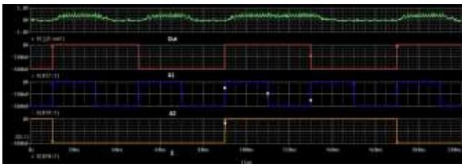
Figure 6: The Output of 2:1 Mux.
