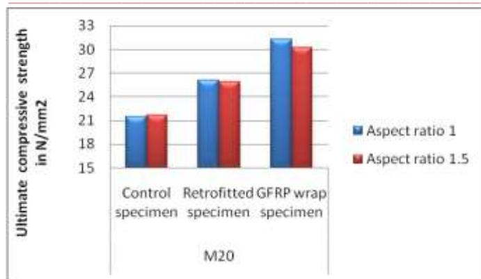
Fig 3 Effect on damaged concrete column retrofitted by GFRP wrap
