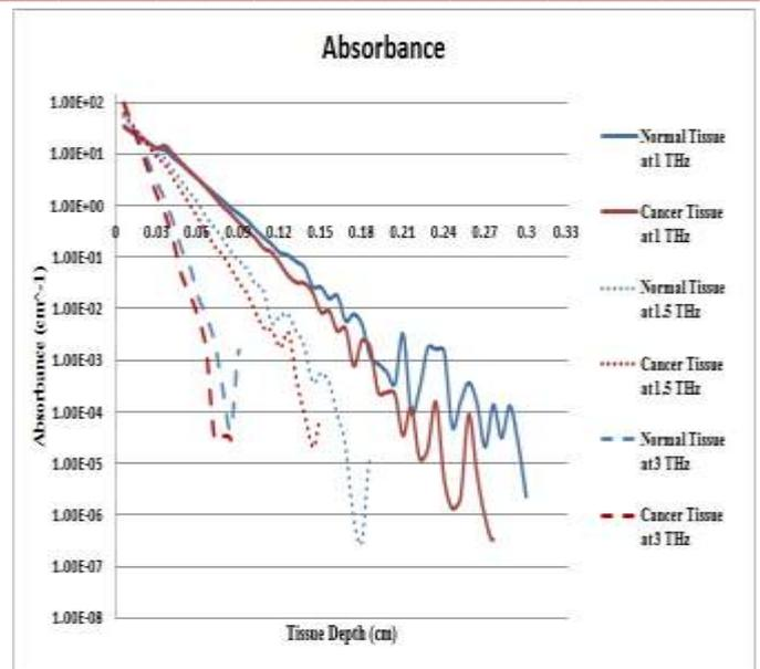
Figure 3: Variation of absorbance based on Tissue depth at various frequencies
