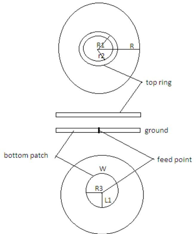
Fig 2: Geometry of the antenna
