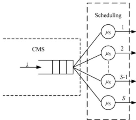
Fig.2.Scheduling subsystem model
