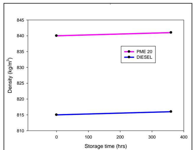
Figure 5: Density vs. storage time.
