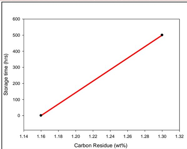
Figure 2: Comparison of the carbon residue of palm-oil biodiesel at various Storage temperatures and times
