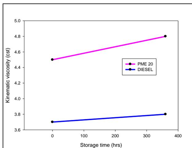
Figure 6: Viscosity vs. storage time at 40 °C.
