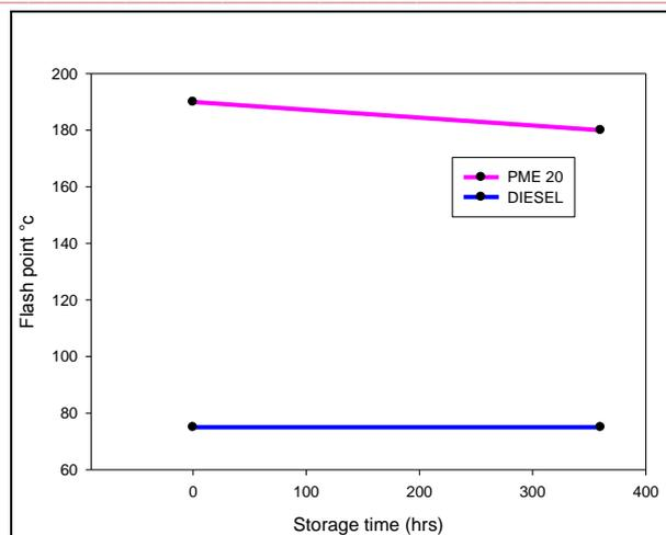
Figure 7: Flash point vs. storage time.
