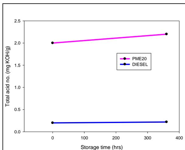
Figure 8: Total acid number vs. storage time.
