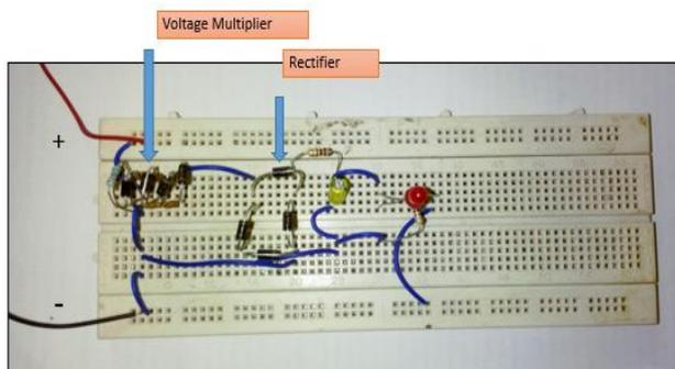
Fig 10. Hardware of the circuit.
