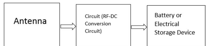
Fig 1. Conceptual block diagram for energy harvesting system.
