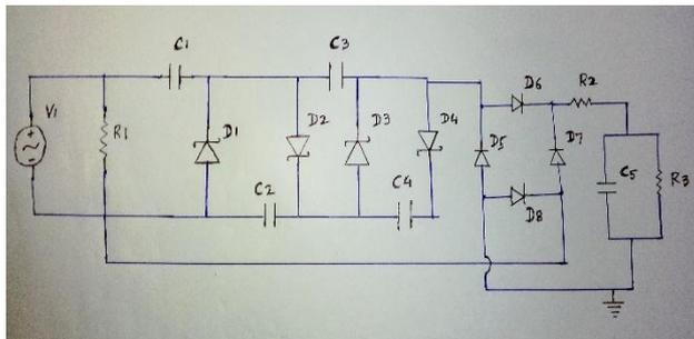
Fig 3. RF-DC Circuit for the system.
