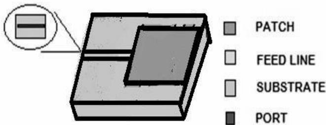
Fig 2. Antenna model square shaped patch design.
