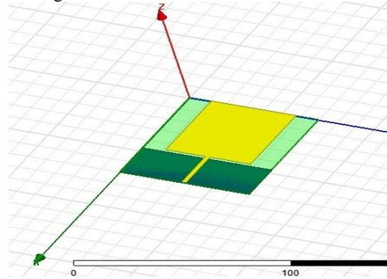
Fig 4. Antenna model using HFSS software.
