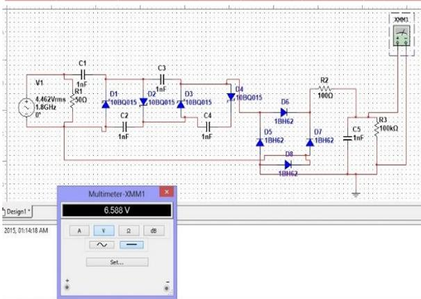
Fig 9. Simulation (DC Voltage) of the circuit at 1.8 GHZ.
