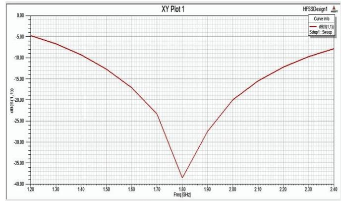
Fig 7. Return Loss of the antenna.
