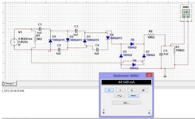
Fig 6. Simulation (DC Current) of the circuit using Multisim Software.
