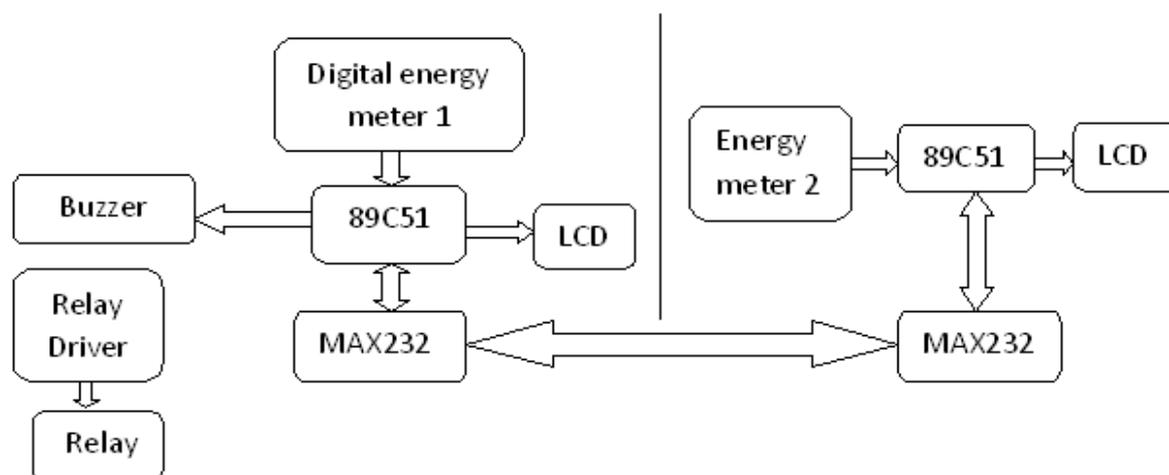
Fig 3: Actual working diagram of Power theft identification.
