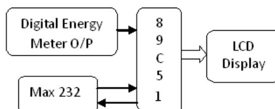
Fig 4: Home side connection of energy Meter (transmitter)
