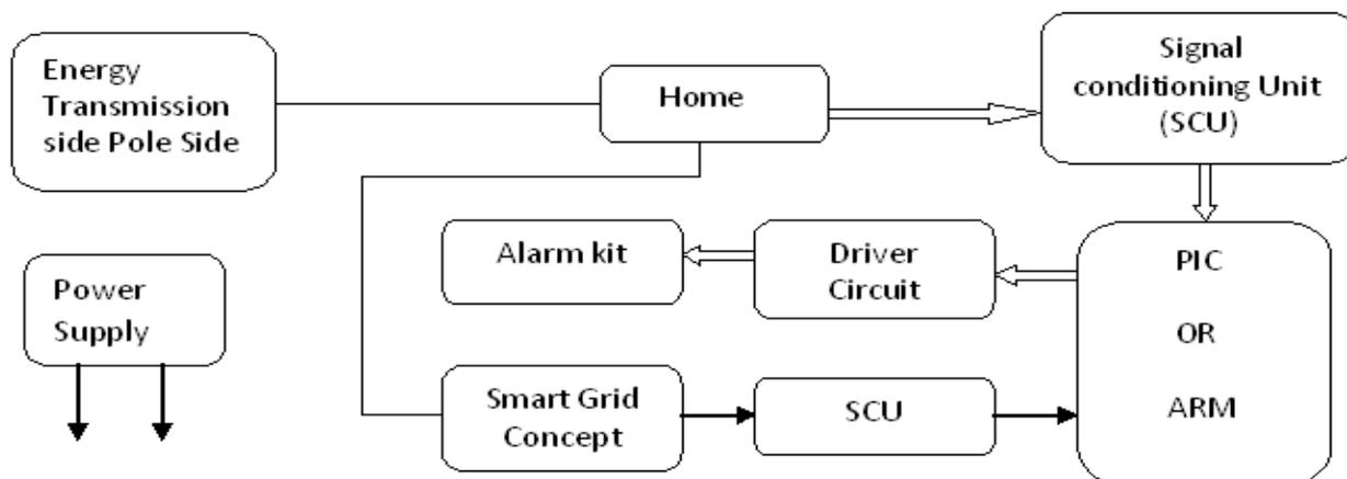
Fig. 2: Block diagram of Power theft identifier using smart grid
