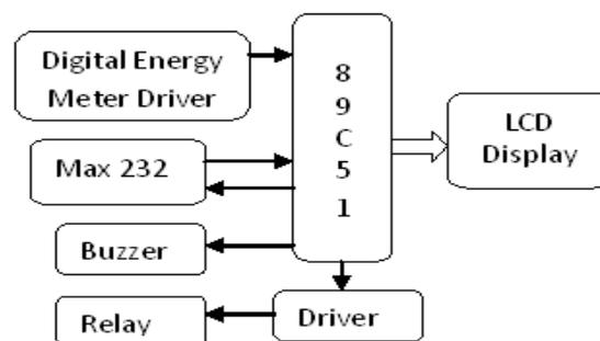
Fig 5: Pole side connection of energy meter (Receiver)
