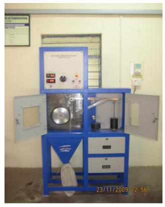
Figure 3: Dry sand abrasive wear testing machine
