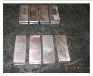
**Figure 1:** Standard test specimen (75×26×6 mm)
