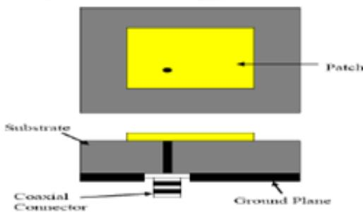
Figure. 3: Coaxial Feed
