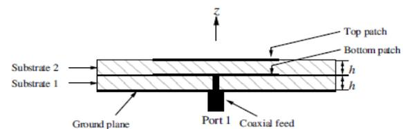
Figure. 1: Micro Strip Patch Antenna Using Broadside Coupling
