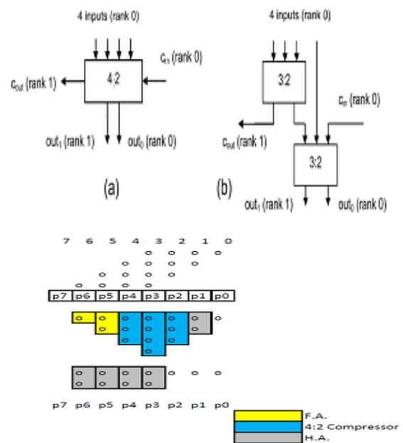
Figure 3. Wallace tree multiplier using 4:2 compressors.
