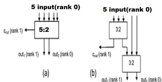
Figure 4. Wallace tree multiplier using 5:2 compressors
