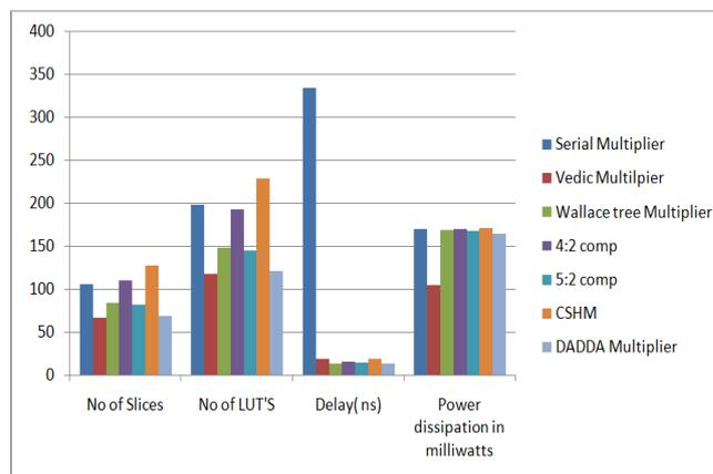
Figure 7. Comparison parameters of different multipliers.
