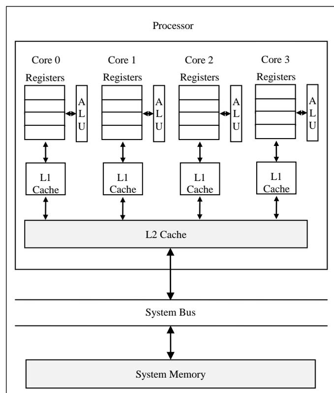
Figure 1 Symmetric Multicore Processor
